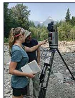
Dr. Piotr Cienciala and geology major McKailey Sabaj use ground-based LiDAR to map deposits of the 2010 Mt. Meager landslide.
