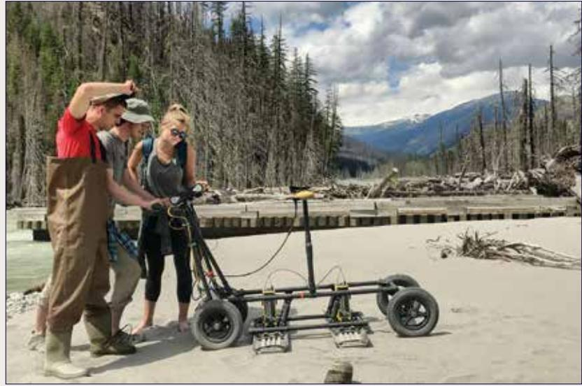
*Students Matt Blaser, Jacob Hesslau, and McKailey Sabaj employ Ground Penetrating Radar to examine the subsurface structure of deposits from the 2010 Mt. Meager Landslide, Pemberton Valley.*
